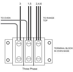
NOTE: 480V UNITS GET WIRED DIRECTLY INTO THE CIRCUIT BREAKER IN THE OVEN, REFER TO WIRING DIAGRAM.
